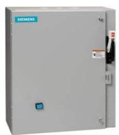
2-speed 3-phase motor starter Size 0 One winding consequent pole Constant or variable torque Solid-state overload relays Low SPD OLR range 0.25-1A High SPD OLR range 5.5-22A 110V 50HZ / 120V 60HZ coil Combination type 25Amp circuit breaker Enclosure NEMA type 4/12 Water/dust tight for outdoors
