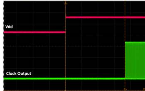
Figure 14. Startup Waveform vs. Vdd
