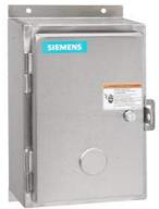
Non-reversing contactor, Size 1 3/4, Three phase full voltage, Contactor amp rating 40A, 3 wire (NO aux included), 110V 50Hz / 120V 60Hz coil, Non-combination type, Encl NEMA type 4X 304 S-Steel, Water/dust tight noncorrosive, Standard width enclosure
