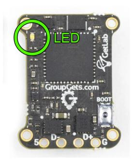
**LED:** When plugged in to power and a Lepton is inserted in the socket LED will flash slowly. When video is being transmitted to the viewing program, LED will flash more rapidly
