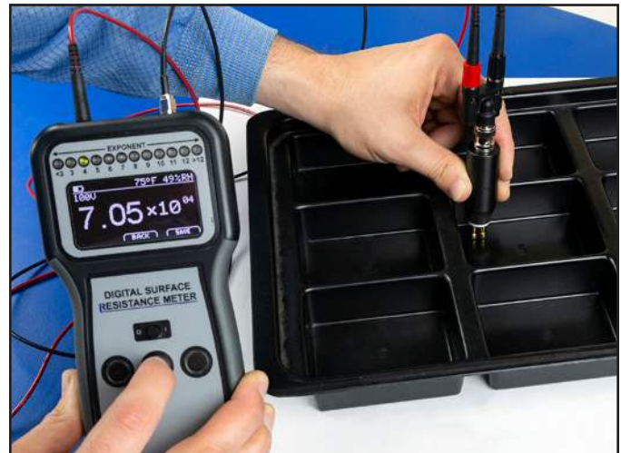
Figure 2. Using the Two-Point Resistance Probe with the Desco 19290 Digital Surface Resistance Meter
