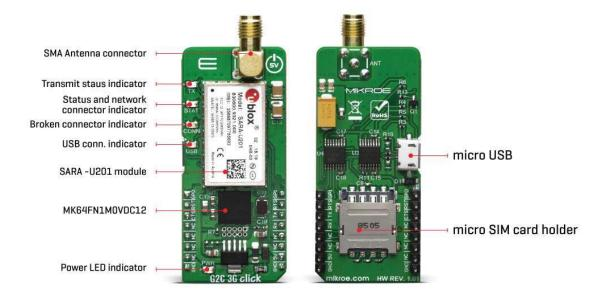
G2C 3G click performs several tasks on its side, which are required to connect to the Click Cloud platform. To establish the connection, an access to a local UMTS/HSPA network with sim card option. For a reliable 3G (UMTS/HSPA) network connection, the Click board™ utilizes the u-Blox SARA U-201 module can be used worldwide.
