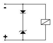
3. When using PWM energy-saving control, ensure that the coil is firstly energized at rated coil voltage for 100mS, the PWM frequency is 20KHz, and duty cycle is > 25%. Similarly, do not directly connect the reverse diodes at both ends of the coil.
