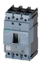
circuit breaker 3VA5 UL frame 125 3-pole, starter protection TM120M, AM, In=90A without overload protection short-circuit protection li=5...12 x In cable connection on both sides
