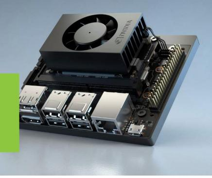
The NVIDIA<sup>®</sup> Jetson Xavier<sup>™</sup> NX developer kit includes a power-efficient, compact Jetson Xavier NX module for AI edge devices. It benefits from new cloud-native support and accelerates the NVIDIA software stack in as little as 10 W with more than 10X the performance of its widely adopted predecessor, Jetson TX2. The capability to develop and test power-efficient, small form-factor solutions with accurate, multi-modal AI inference opens the door for new breakthrough products.
