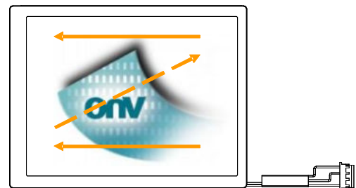
Fig. 2 Reverse scan (Pin4, DPS = High)
