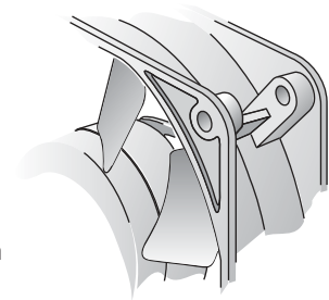
Series 8000 A with reinforced flanges
