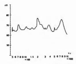
applied voltage: 1.5 V, 1/2 duty, square wave distance for measurement: 10 cm
