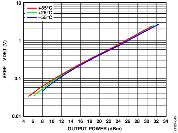
Figure 45. Detector Voltage (VREF - VDET) vs. Output Power for Various Temperatures at 32 GHz
