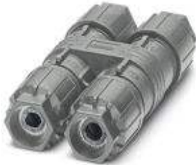
QUICKON H-distributor, gray, 4-pos. without PE, 1.0 mm 2 ... 2.5 mm 2 / 630 V / 20 A, for cable diameters of 6 mm ... 10 mm, with a sealing bolt.
