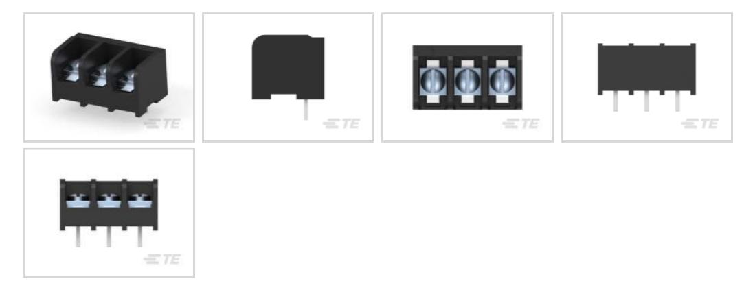
Barrier Strip Style: Tri-Barrier Bottom Termination Type: Printed Circuit Pin Connector System: Wire-to-Board Number of Positions: 3 Centerline (Pitch): 9.53 mm [.375 in ]
