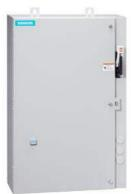
Reversing motor starter, Size 0, Three phase full voltage, Solid-state overload relay, OLR amp range 0.75-3.4A, 24VAC 50-60Hz coil, Combination type, 3A circuit breaker, Encl NEMA type 4X 304 S-Steel, Water/dust tight noncorrosive
