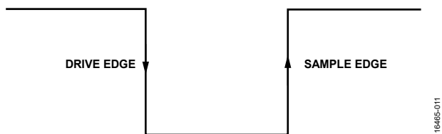
Figure 32. SPI Mode 3 SCLK Edges
