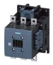
power contactor, AC-3 265 A, 132 kW / 400 V AC (50-60 Hz) / DC operation 23-26 V AC/DC auxiliary contacts 2 NO + 2 NC 3-pole, frame size S10 busbar connections drive: conventional spring-loaded terminal
