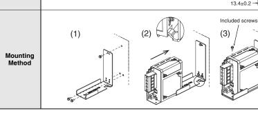
Recommended tightening torque M3: 0.54 N·m
