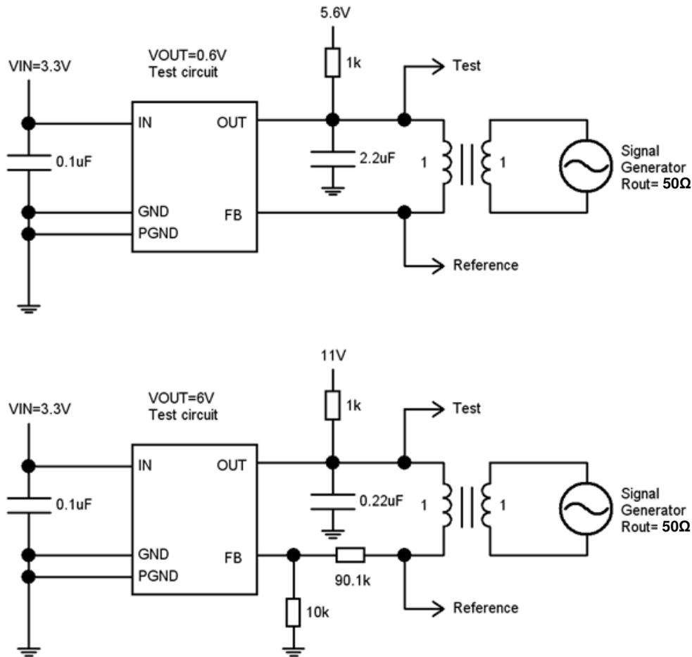
Fig. 2 Test Circuits for Gain and Phase Plots
