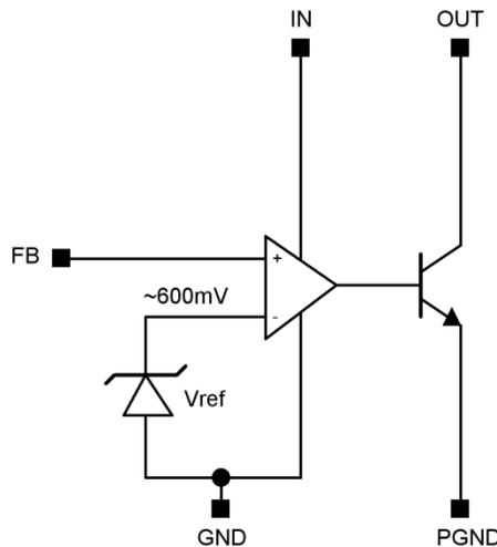
The ZXRD060 differs from most other shunt regulators in that it has separate input and output pins and a low voltage reference. This enables it to regulate rails down to 600mV and makes the part ideal for isolated power supply applications that use opto-couplers in the feedback loop and where the open-collector output is required to operate down to voltages as low as 200mV.
