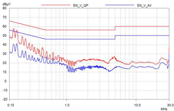
Figure 26 – Floating Ground EMI (Neutral), 20 V / 100% Load for 230 VAC.
