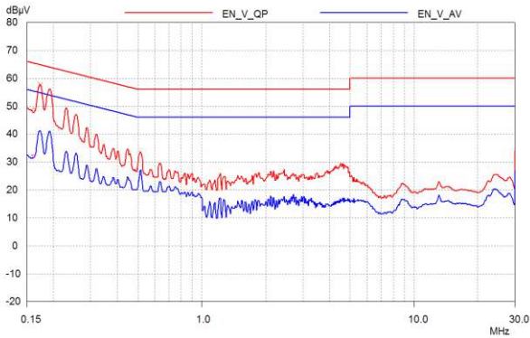
Figure 30 – Earth Ground EMI (Neutral), 20 V / 100% Load for 230 V AC.
