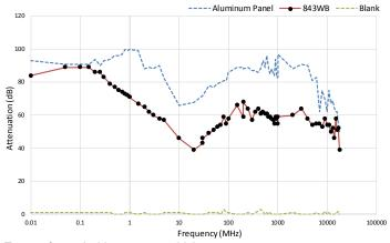
Test performed with a two-coat thickness.
