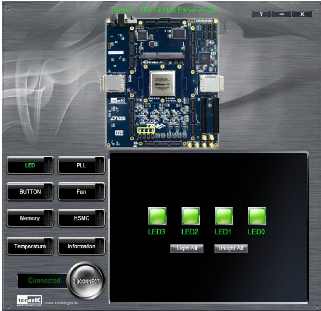
Figure 3-2 TR4 Control Panel is Ready
