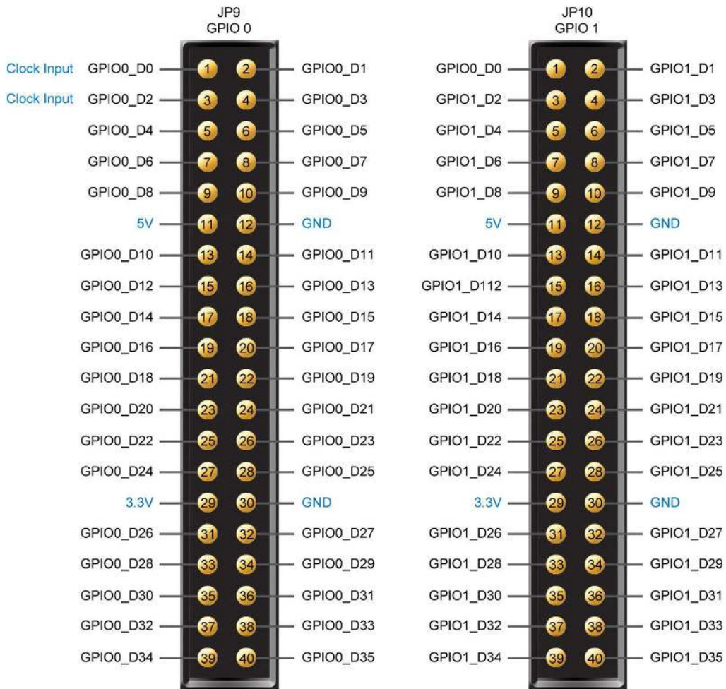
Figure 2-21 Pin Distribution of the GPIO Expansion Headers
