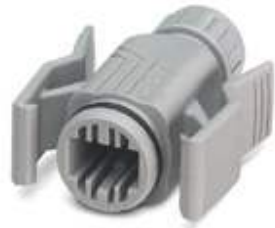
RJ45 sleeve housing, IP67, for pin insert VS-08-ST-RJ45, with push-pull interlocking for panel mounting frames, for cable cross section 5.0 mm ... 6.5 mm
