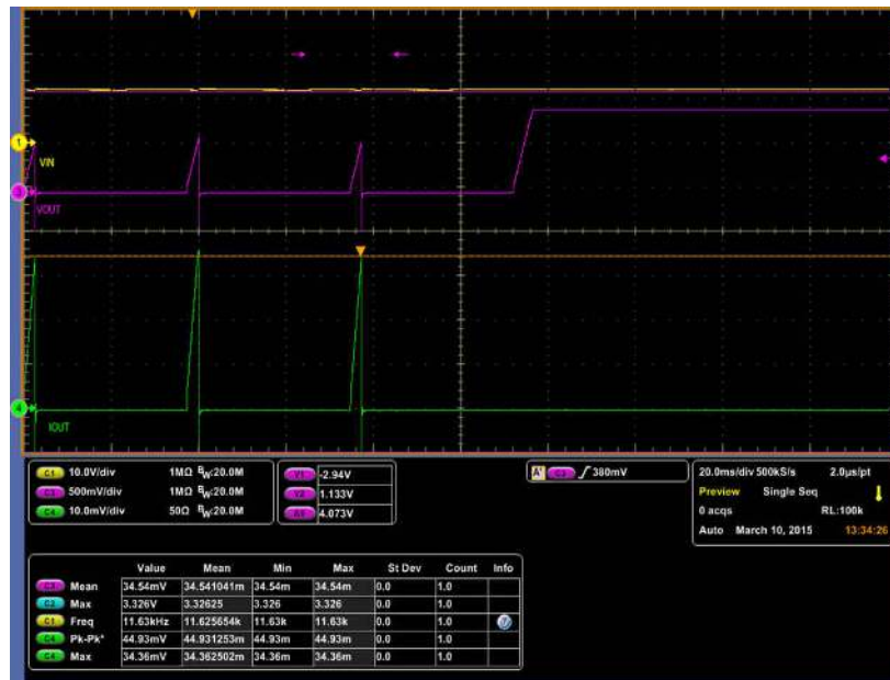
Figure 8-11. Restart from Overcurrent Protection, 0.95-V Output at 12 V_{IN}
