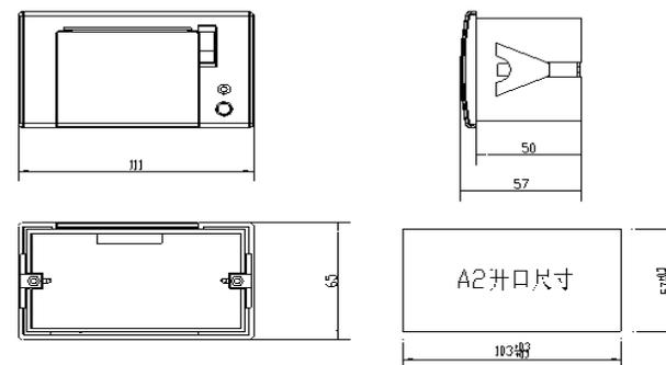
**Model No.: A2 Micro Panel Thermal Printer**
