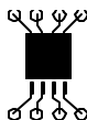
b) 105^\circ\text{C}/\text{W} when mounted on a .04\text{ in}^2 pad of 2 oz copper
