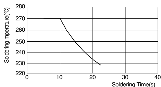
[Allowable Flow Soldering Temperature and Time]
