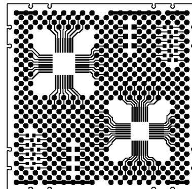
Supports 36 pins with a .5mm pitch and 32 pins with a .65mm pitch for QFN devices
