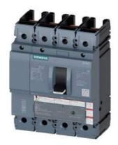
circuit breaker 3VA5 UL frame 250 breaking capacity class C 100kA @ 480V 4-pole, line protection TM210, FTFM, In=125A overload protection Ir=125A fixed short-circuit protection Ii=10 x In N conductor unprotected without connection
