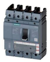
circuit breaker 3VA5 UL frame 250 breaking capacity class M 35kA @ 480 V 4-pole, line protection TM230, FTAM, In=175A overload protection Ir=175A fixed short-circuit protection Ii=5...10 x In N conductor protection 100% without connection
