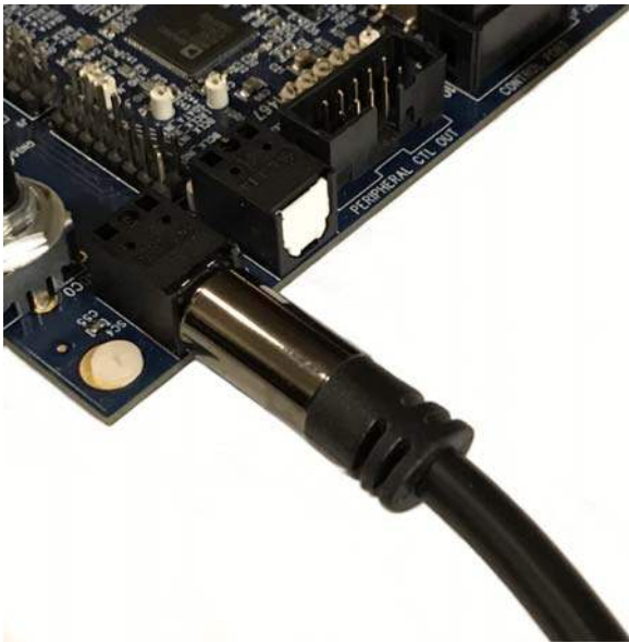
Figure 35. Photograph of the Optical S/PDIF Input Connection
