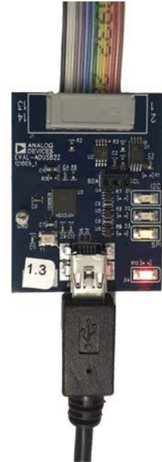
Figure 7. State of the USBi Status LEDs After Driver Installation
