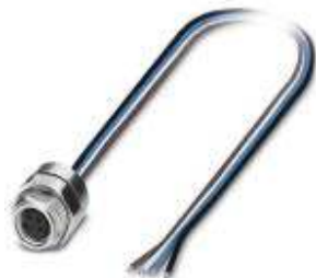
Sensor/actuator flush-type socket, 4-pos., M8, rear/screw mounting with M12 thread, with 0.5 m TPE litz wire, 4 x 0.25 mm 2
