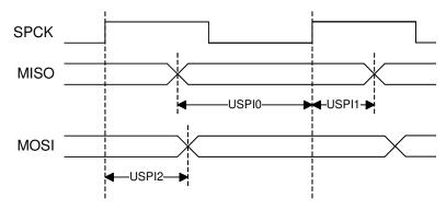
**Figure 9-8.** USART in SPI Master Mode with (CPOL= 0 and CPHA= 1) or (CPOL= 1 and CPHA= 0)
