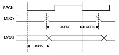
USART0 in SPI Mode Timing, Master Mode<sup>(1)</sup> Table 9-54.
