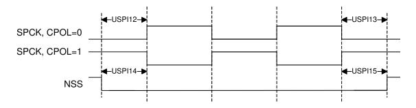
Table 9-58. USART0 in SPI mode Timing, Slave Mode<sup>(1)</sup>
