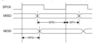
Figure 9-13. SPI Master Mode with (CPOL= 0 and NCPHA= 1) or (CPOL= 1 and NCPHA= 0)
