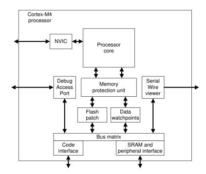
The Cortex-M4 processor is built on a high-performance processor core, with a 3-stage pipeline Harvard architecture, making it ideal for demanding embedded applications. The processor delivers exceptional power efficiency through an efficient instruction set and extensively optimized design, providing high-end processing hardware including a range of single-cycle and SIMD multiplication and multiply-with-accumulate capabilities, saturating arithmetic and dedicated hardware division.
