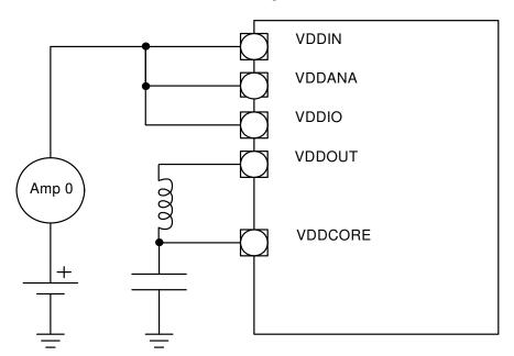
Figure 9-2. Measurement Schematic, Switching Mode
