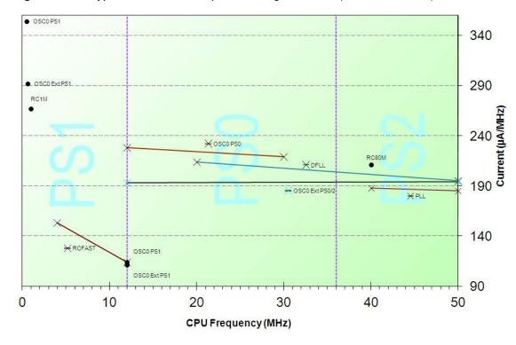
**Figure 9-1.** Typical Power Consumption running Coremark (from above table)
