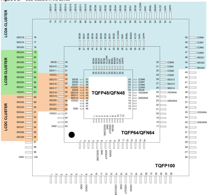
Figure 6-5. LCD clusters in the device
