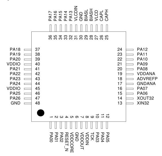
Figure 3-5. ATSAM4LC TQFP48/QFN48 Pinout
