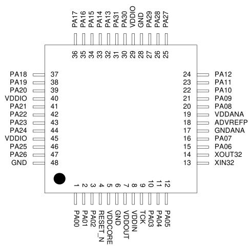
Figure 3-10. ATSAM4LS TQFP48/QFN48 Pinout
