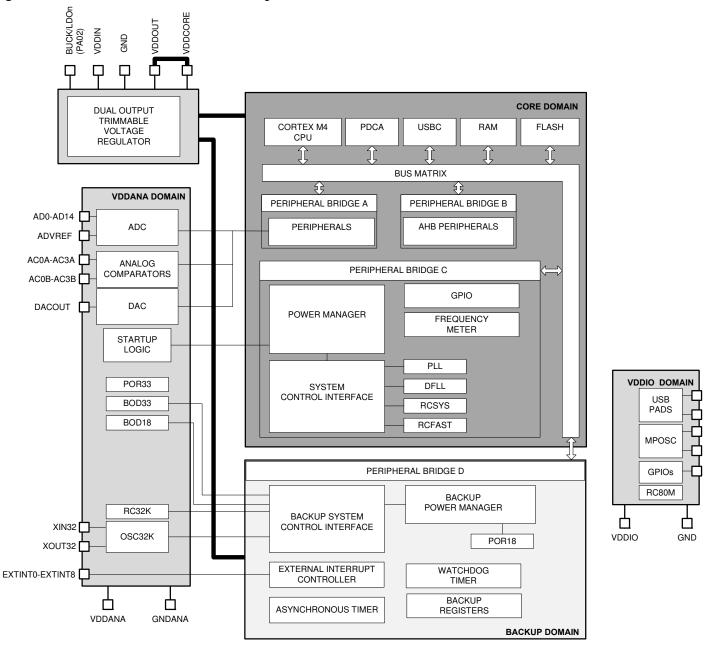
Figure 6-2. ATSAM4LC Power Domain Diagram
