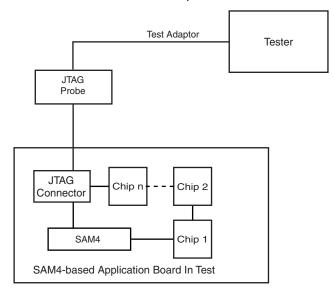
Figure 8-9. Application Test Environment Example
