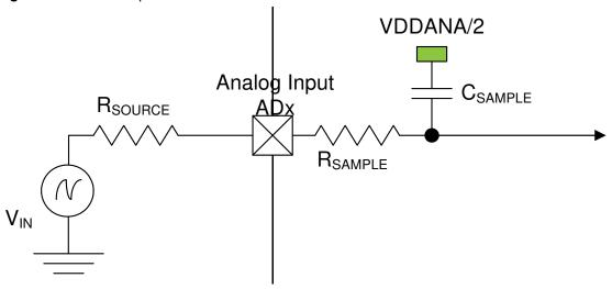
To achieve n bits of accuracy, the  $C_{SAMPLE}$  capacitor must be charged at least to a voltage of  $V_{CSAMPLE} \ge V_{IN} \times (1-2^{-(n+1)})$
