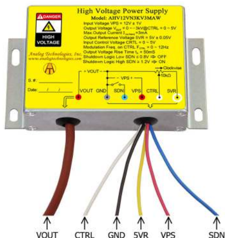
Figure 2. The Connecting Lead Wires of AHV12VN3KV3MA
