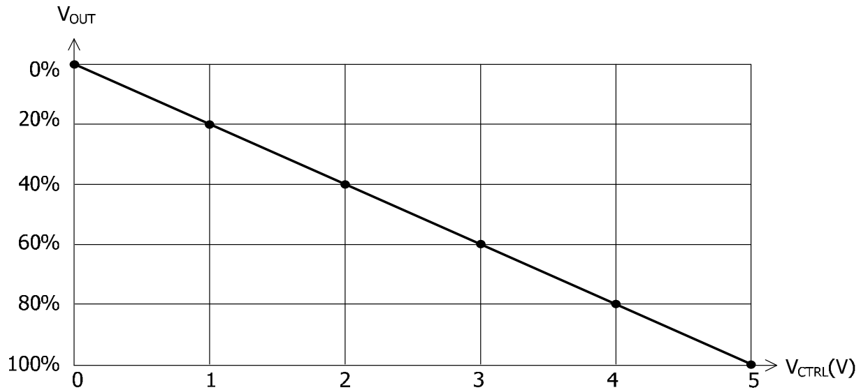
Figure 7. V_{CTRL} vs. V_{OUT}
