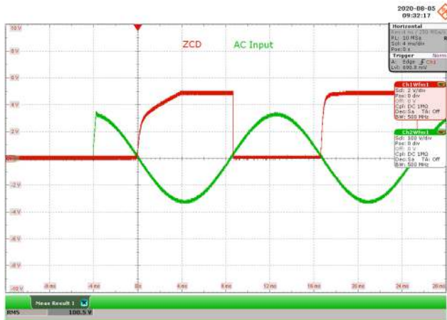
Figure 27 – 115 VAC 60 Hz, No Load CH1: ZCD, 2 V / div., 4 ms / div. CH2: V_{IN} , 100 V / div., 4 ms / div.
