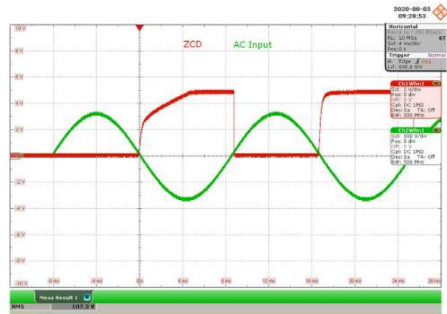
Figure 24 – 115 VAC 60 Hz, Full Load CH1: ZCD, 2 V / div., 4 ms / div. CH2: V IN , 100 V / div., 4 ms / div.
