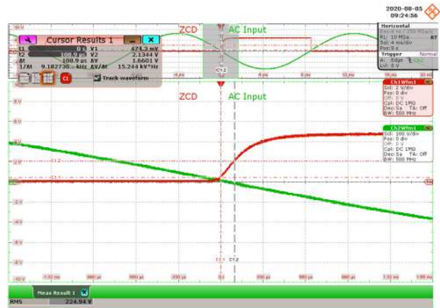
Figure 34 – 230 VAC 50 Hz, Full Load. CH1: ZCD, 2 V / div., 4 ms / div. CH2: V_{IN} , 100 V / div., 4 ms / div. Rising edge delay = 100.9 μs.
