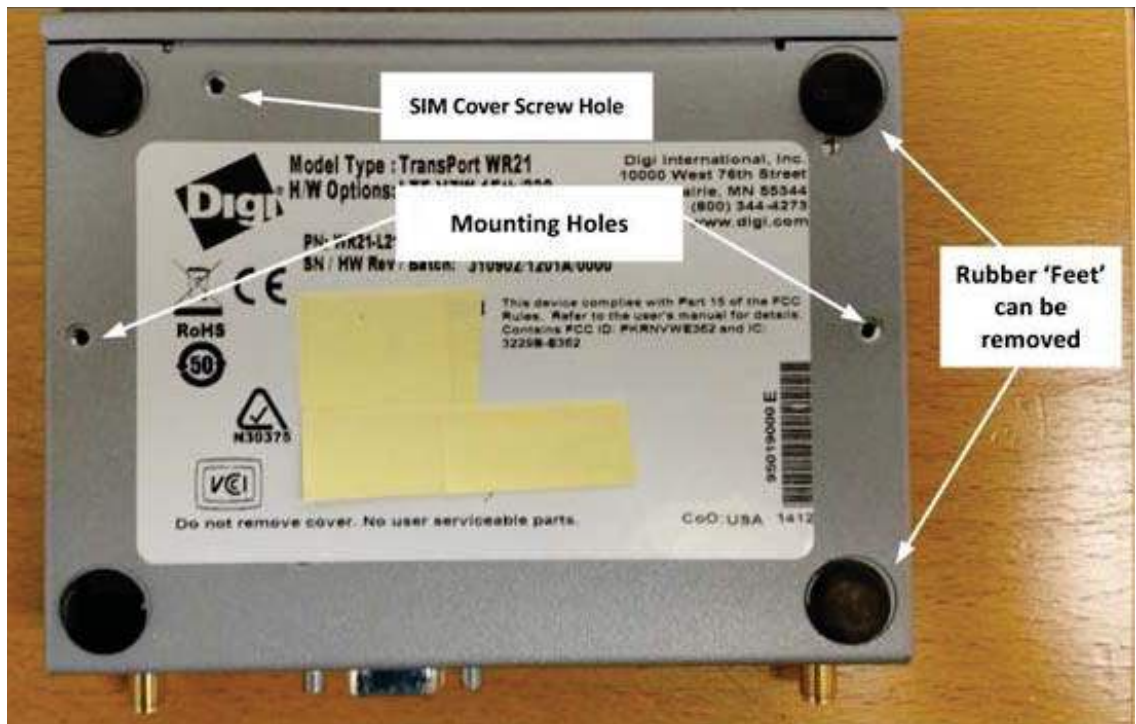
Bottom view of a Digi TransPort WR21.
