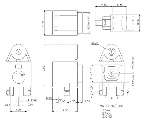
Note: 1.All dimensions are in millimeters.2.General Tolerance: ±0.3mm
