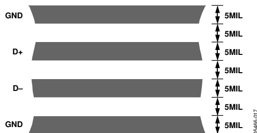
Figure 22. Typical Arrangement of Signal Tracks
