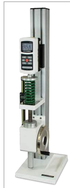
Shown with a TSF test stand in a spring testing application
