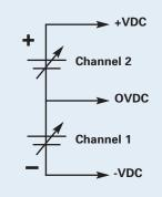
This feature is useful for powering bipolar circuits and devices.
