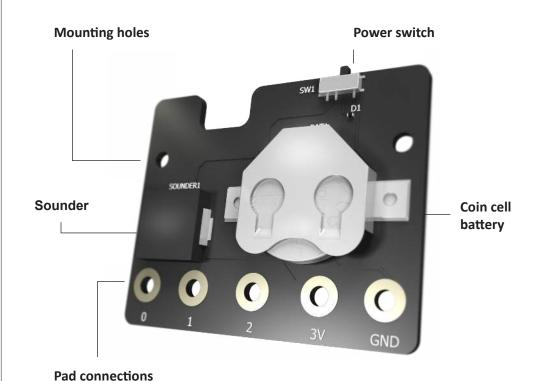
**Technical information:** The included CR 2032 Lithium battery has a capacity of 200mAh which depending on use should last up to 20 hours. The on-board sounder can output frequencies from 200Hz to 10kHz at volumes over 75dB! The sounder is connected to P0. P1 and P2 are not used.
