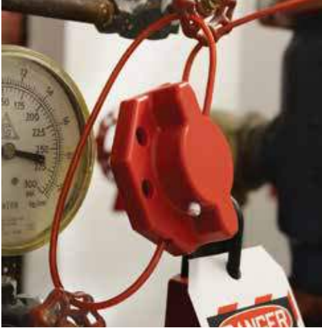
Turn the hasp halves to cinch cable.
