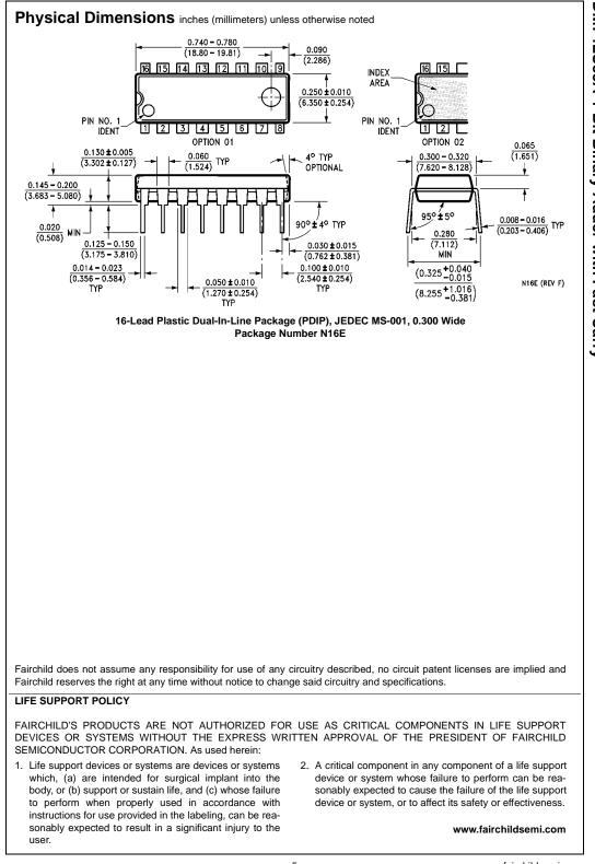
DM74LS83A 4-Bit Binary Adder with Fast Carry
