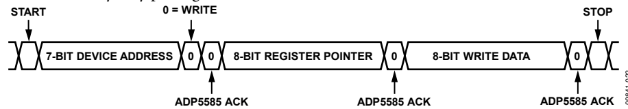
Figure 23. I 2 C Single Byte Write Sequence
