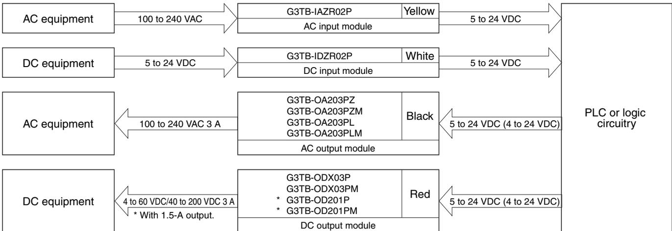
• When mounting more than one output module, make a distance of 5 mm minimum between adjacent SSRs. Up to 16-point, 3-A load switching is possible.
