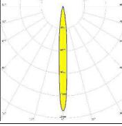
LED LH351Z FWHM / FWTM 11.0° / 19.0° Efficiency 89 % Peak intensity 20.7 cd/lm LEDs/each optic 1 White Light colour
