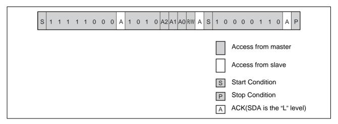
Even if the MB85RC64TA stays in the Sleep mode, SDA and SCL signals are monitored. Following sequences enable the transition to Standby mode after recovery time (tree) of internal regulator circuits.
