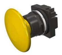
30mm BlackMax, Epoxy Coated Corrosion Resistant Metal Operator, Round Push-Pull Operator Non-Illuminated Mushroom Head Cap Large 2 1/2" (63.5 mm) Plastic, Yellow 3 Position Momentary UL Listed, CSA Certified NEMA 1,3,3R,4,4X,12,13 & Automotive Standards
