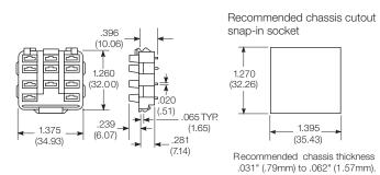
Hard mount sockets for relays with 4 poles Socket with printed circuit terminals is available for KUP relays, with 4 poles, with .110" (2.79mm) quick connect terminals. 27E043-with solder eyelet terminals. 27E419-with printed circuit terminals.
